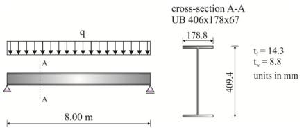
Figure 1: Simply supported steel beam
