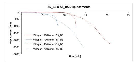
Figure 4: Midspan displacement for case SS\_B3 and SS\_B5
