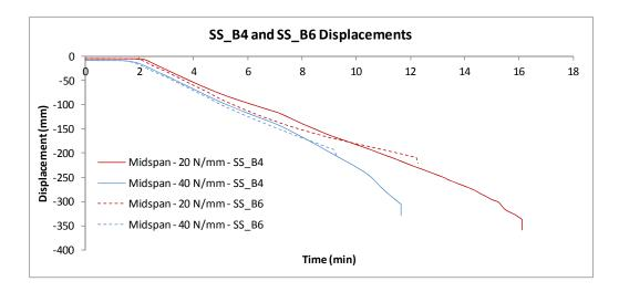
Figure 5: Midspan displacement for case SS\_B4 and SS\_B6
